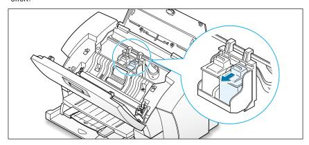
5. Lift the cartridge up and out of the cartridge holder.
